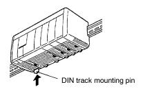
5. Install a DIN Track Bracket on each side of the PC. To install a bracket, hook the bottom of the Bracket on the bottom of the track, rotate the Bracket to hook the top of the Bracket on the top of the track, and then tighten the screw to lock the Bracket in place.
